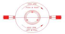
Nozzle Adjustment for 4000 US GPM / 2000 US GPM
