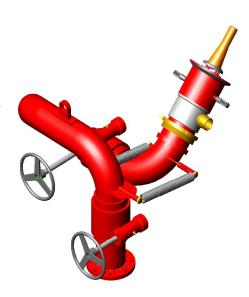
bearing for rotation in horizontal and vertical direction through hand wheel operation even under high operating pressures. The monitor assembly is designed to withstand the nozzle reaction force experienced during the operation of jet/ fog.
